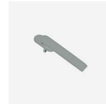
Flat handle for bi-fold systems Ref. A0023400 7 mm spindle 60 mm escutcheon
