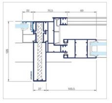
Cross-section fixed structure - outward
